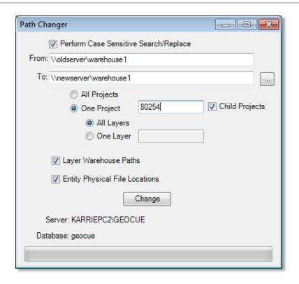
7. The tool performs a simple text replacement in the physical file paths of the GeoCue database. It performs a direct substitution of the 'From' string with the 'To' string leaving the rest of the path intact, so set the "From" and "To" fields appropriately. Here are some basic examples:
