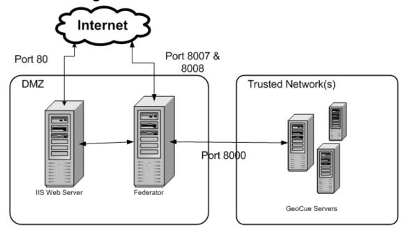
In this configuration, the IIS Web Server and the Federator are on a Demilitarized Zone (DMZ) network. The GeoCue Servers are connected to the trusted network(s). If you want to be able to access the web applications (Federator Admin, Federator User Manager, and Federator License Manager) from outside you network(s), you will need to open a few ports to allow communication.
