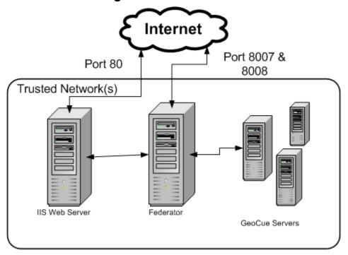
In this configuration, all the servers (IIS Web Server, Federator, and GeoCue Servers) are connected to the same network or to multiple trusted networks. If you want to be able to access the web applications (Federator Admin, Federator User Manager, and Federator License Manager) from outside you network(s), you will need to open a few ports to allow communication.
