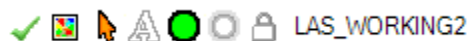
Figure 2 - Layer in TOC showing Production State turned on for the visible and selectable layer
