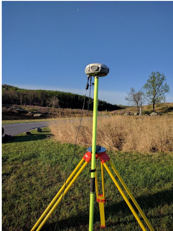
Figure 3 - GNSS base station
