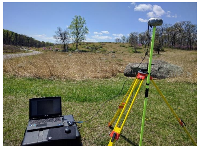
Figure 7 - eBee control station - laptop connected to GNSS base station
