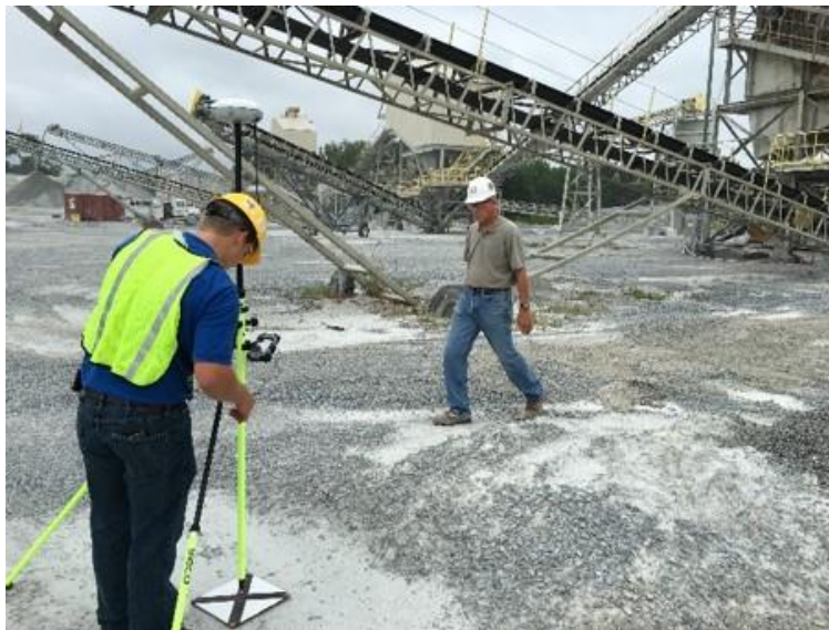
Figure 3: Setting a "homemade" ceramic tile GCP
