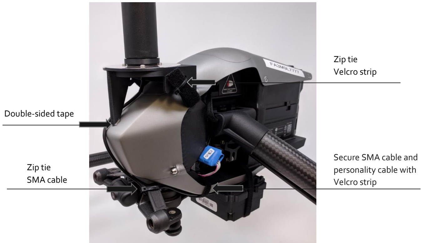
Inspire 2 - Antenna and personality cable routing and installation
