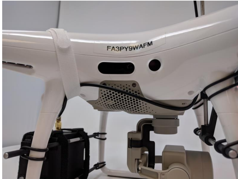
Phantom 4 Pro – SMA cable routing
