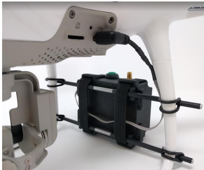
Phantom 4 Pro – Personality cable routing
