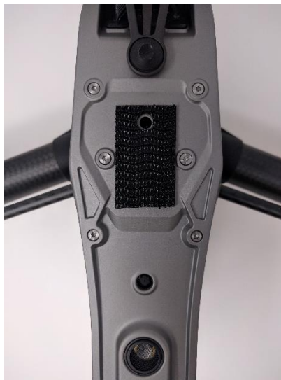
Inspire 2 and Loki controller – Velcro positioning
