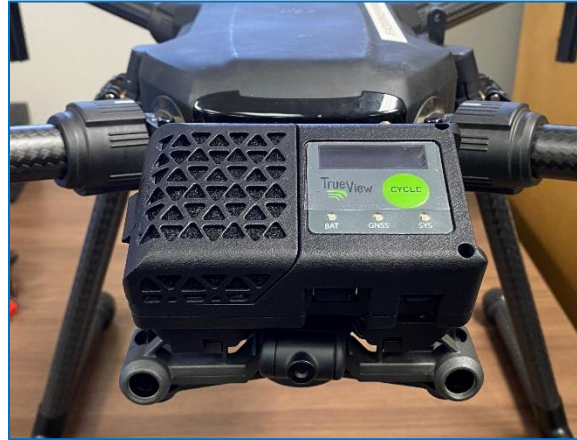
Figure 16 - Controller Box attached to Controller Box Plate
