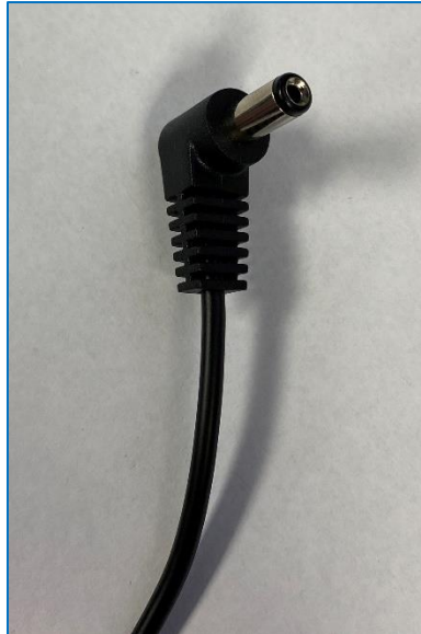
Figure 15 - Power Cable with Doubled Ended Barrel Connectors
