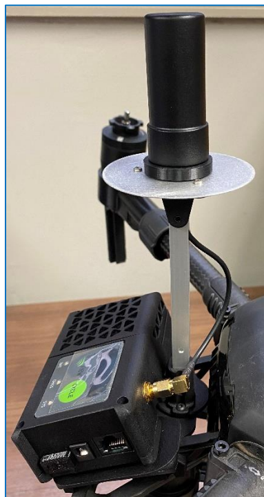
Figure 17 - GNSS Antenna and Mast
