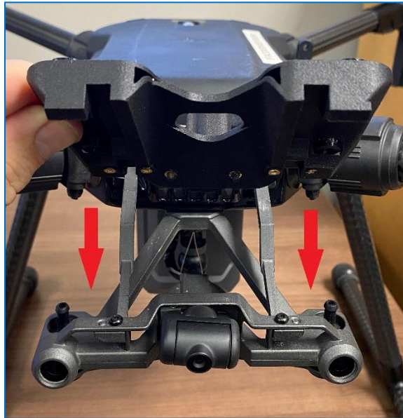
Figure 6 - Place Control Box Plate on Skyport Assembly
