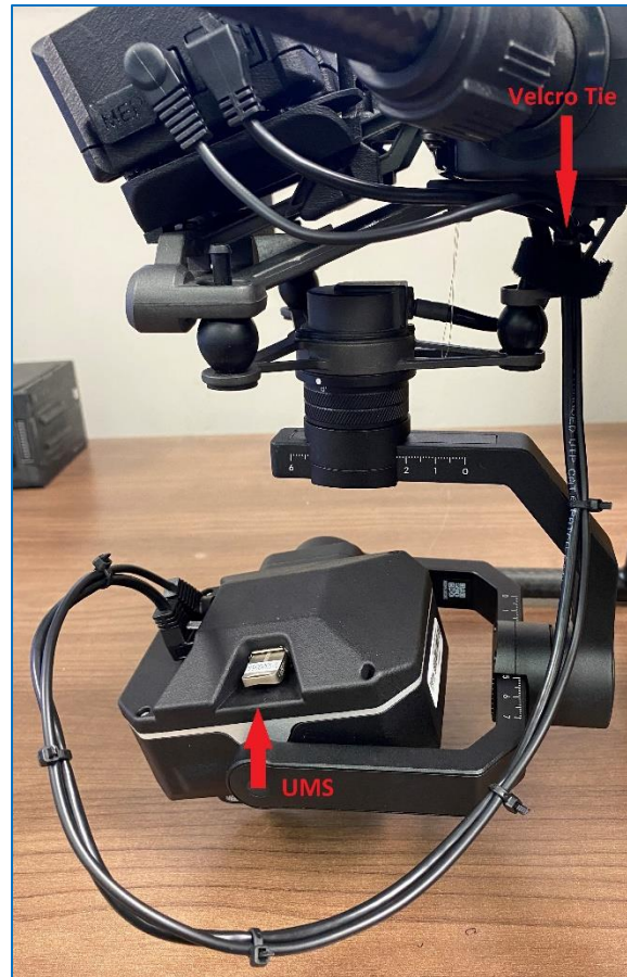
Figure 19 - Cable management and UMS
