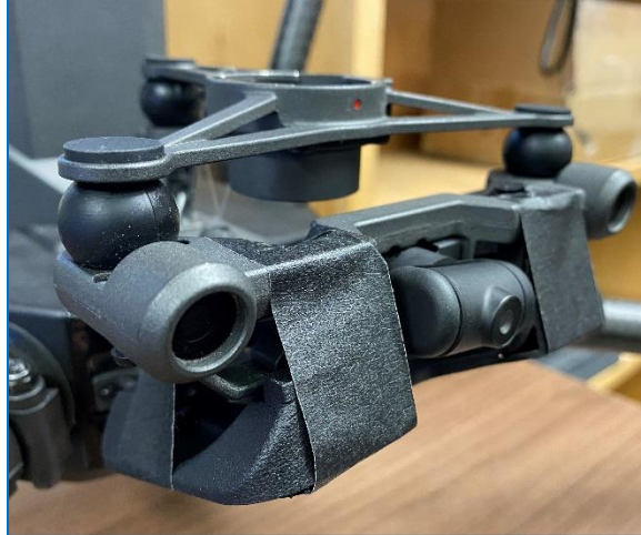
Figure 7 - Masking Tape Securing the Controller Box Plate
