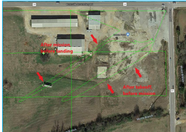
Figure 49 - Heading Alignment Maneuver
