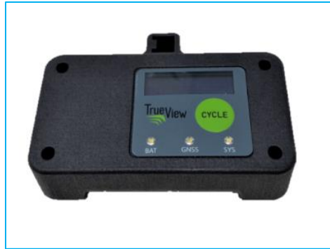
Figure 3 - Controller Box with readout display
