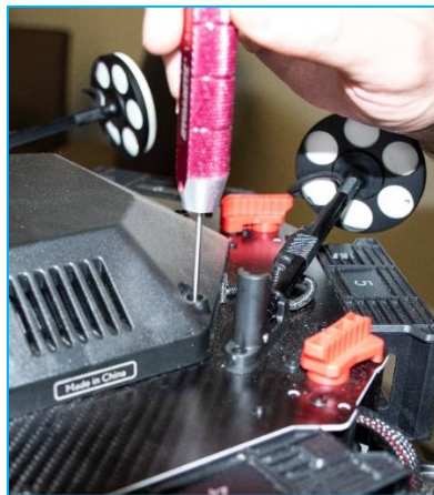
Figure 8 – Install set screws
