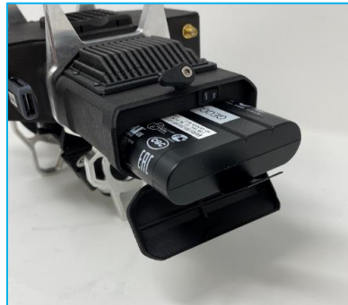
Figure 41 – Insert TrueView Battery
