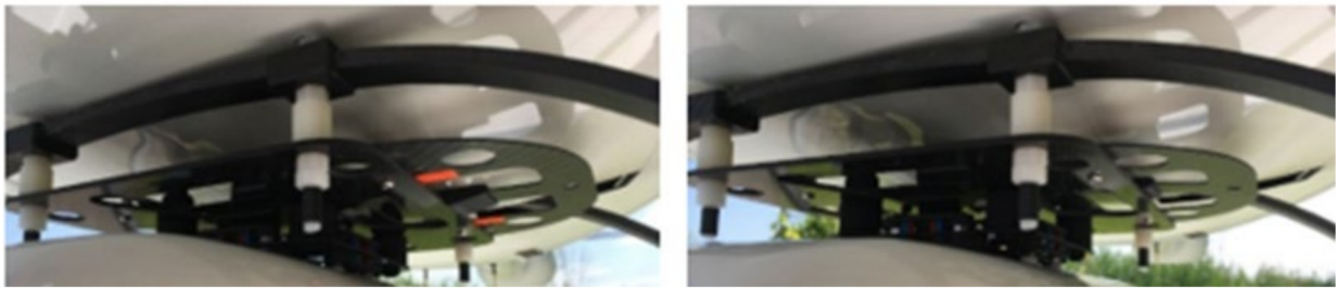
Figure 16. Make sure the payload clips are in the fully extended position. Confirm that there are no orange arrows showing on the adapter clip.
