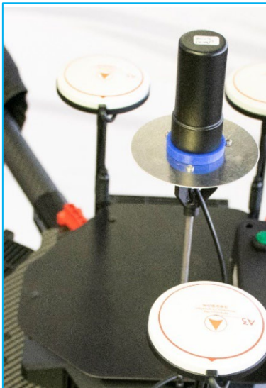
Figure 24. GNSS antenna installed on DJI M600.
