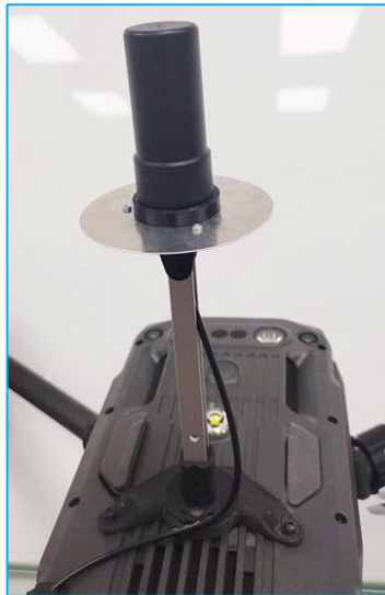
Figure 25. AV14 GNSS antenna installed on M300.
