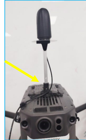
Figure 33. AV18 GNSS antenna installed on M300.
