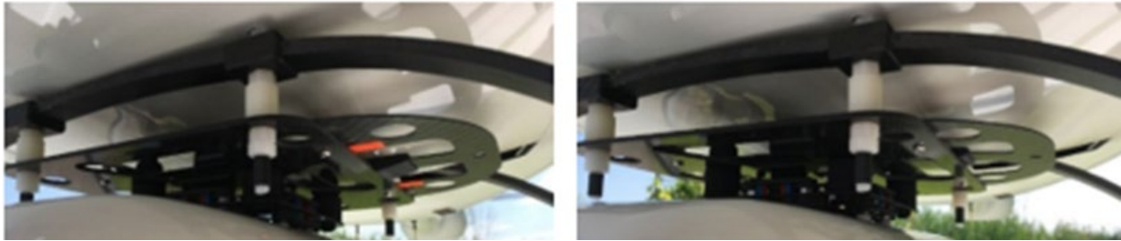
Figure 14. Make sure the payload clips are in the fully retracted position. Confirm that there are no orange arrows showing on the adapter clip.
