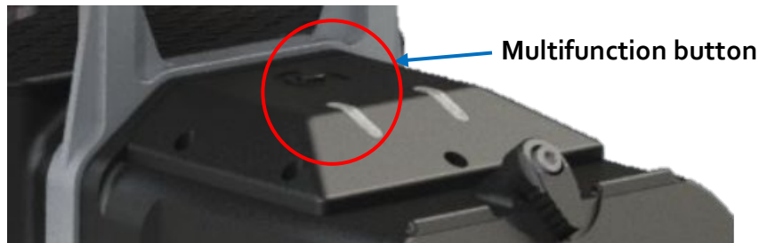
Figure 7. Multifunction button located at the top of the battery compartment of the payload.
