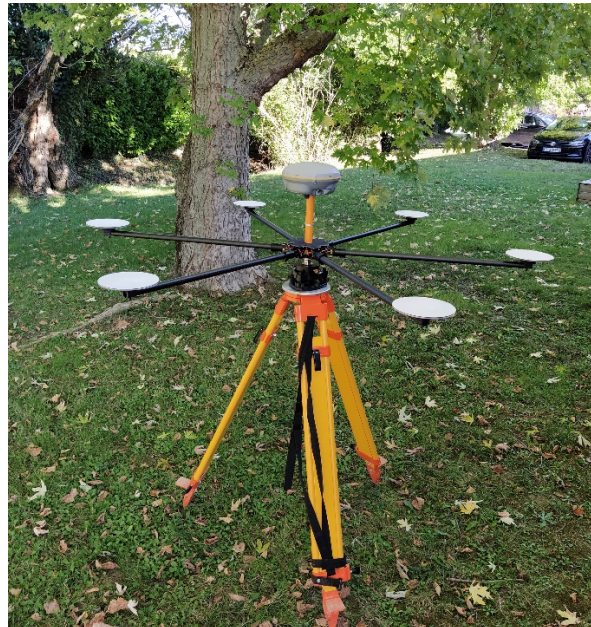
Figure 4: Accuracy star installed on a tripod with a GNSS receiver at the center. The reference position of the GCP is given by GNSS processing. The reflectors are used to compute the geometric center of the hexagon from the LiDAR point cloud.
