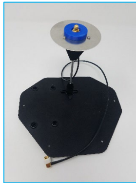
Figure 1. Top plate with antenna mast.
