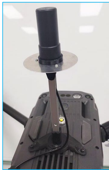
Figure 25. AV14 GNSS antenna installed on M300.
