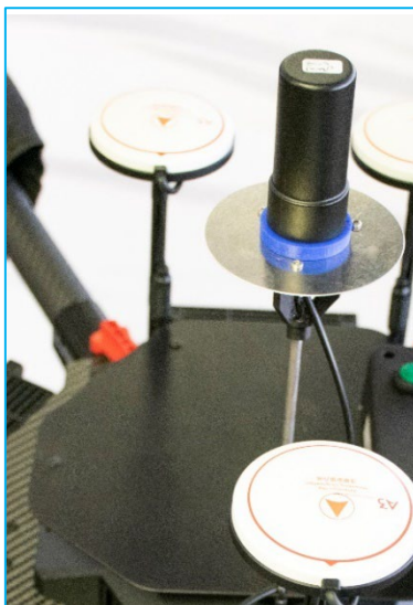
Figure 24. GNSS antenna installed on DJI M600.
