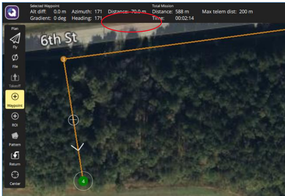
Figure 28: Distance from Waypoint 3 to Waypoint 4 is shown at the top left of the window.
