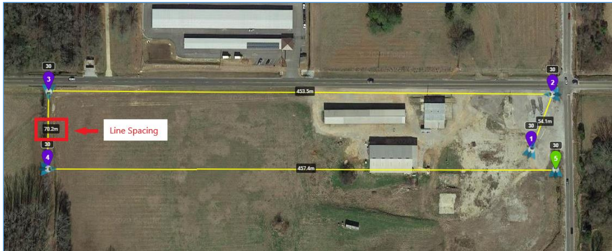
Figure 10 – Line Spacing in Mission Hub
