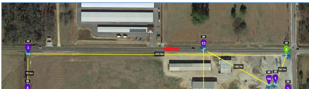
Figure 12 – Linear descent between waypoints
