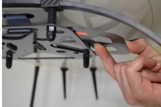
Figure 15. Release the adapter clip.
