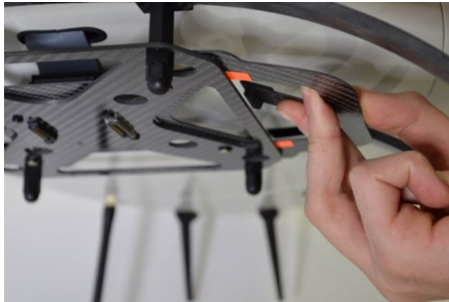
Figure 17. Release the payload adapter clip.
