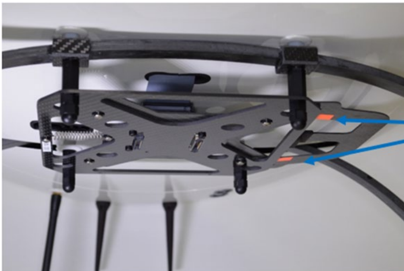
Figure 14. Orange safety arrows on the payload adapter clip (open position).
