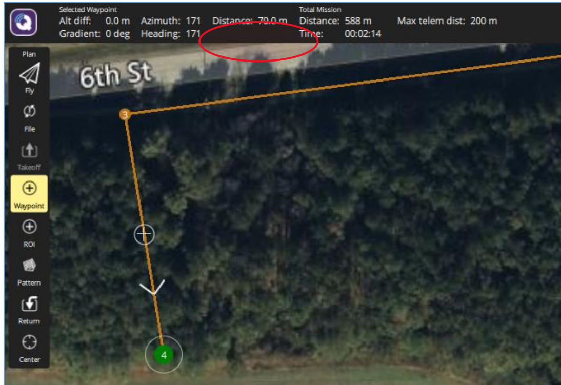
Figure 28: Distance from Waypoint 3 to Waypoint 4 is shown at the top left of the window.
