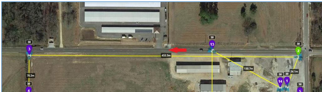
Figure 12 – Linear descent between waypoints
