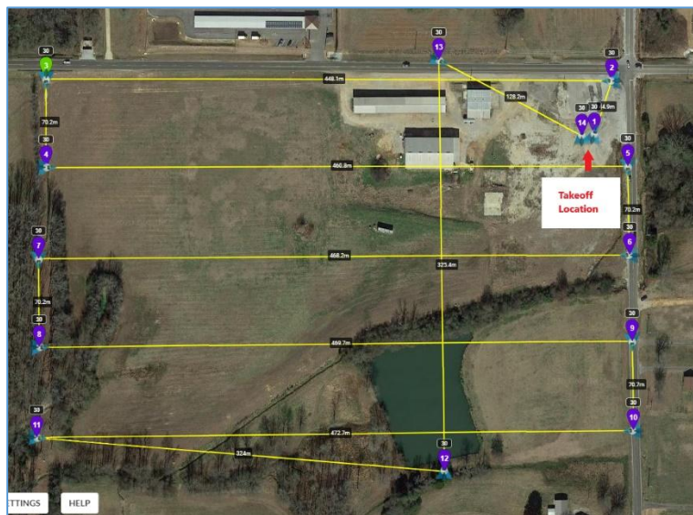
Figure 11 – Set the final waypoint to the takeoff location. Flight plan illustrates North/South control/cross strip included.
