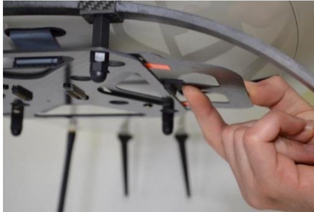
Figure 11. Release the adapter clip.
