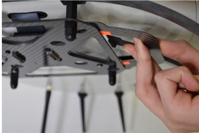
Figure 13. Release the payload adapter clip.
