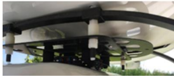
Figure 12. Make sure the payload clips are in the fully retracted position. Confirm that there are no orange arrows showing on the adapter clip.
