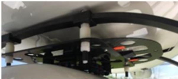
Figure 12. Make sure the payload clips are in the fully retracted position. Confirm that there are no orange arrows showing on the adapter clip.
