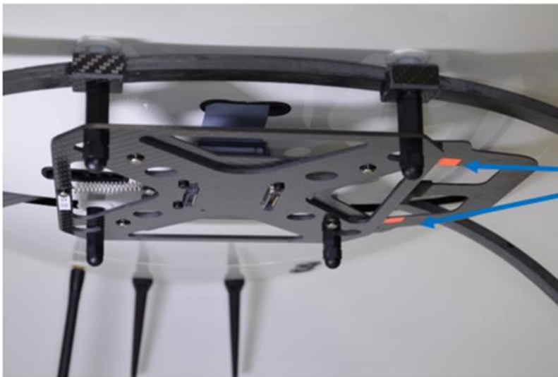
Figure 10. Orange safety arrows on the payload adapter clip (open position).
