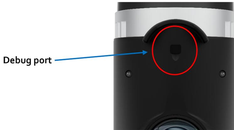
Figure 8. Debug port is located at the bottom right side of the payload.
