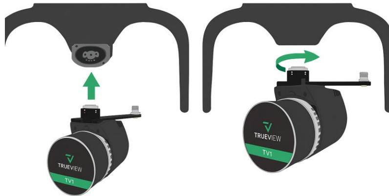
**Figure 17 DJI Skyport Interface Payload Installation**
