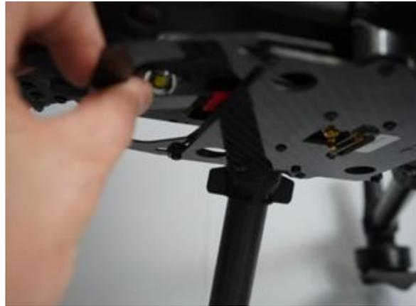
Figure 16. Release the payload adapter clip.
