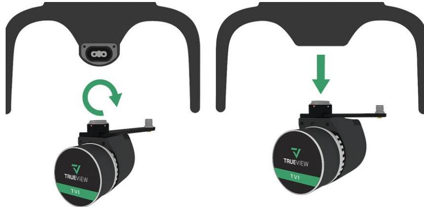
**Figure 18 DJI Skyport Interface Payload Release**
