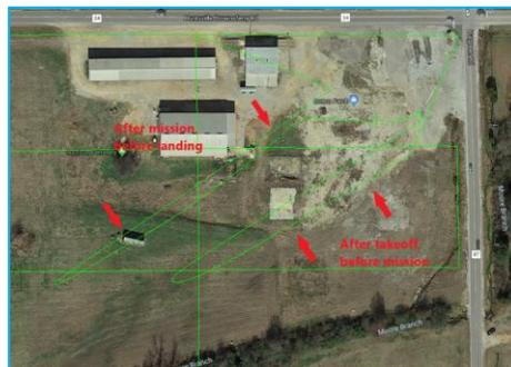
**Figure 20. Heading alignment maneuver.**
