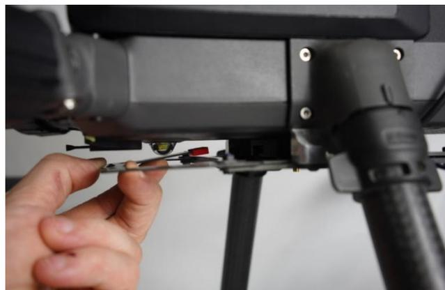
**Figure 14. Release the adapter clip.**
