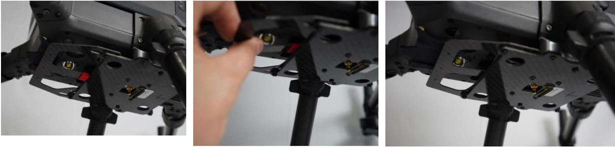
Figure 15. Make sure the payload clip is in fully retracted position. Confirm orange tab is no longer visible.
