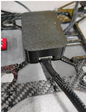
Figure 6 - Plug the power cable into the payload adapter
