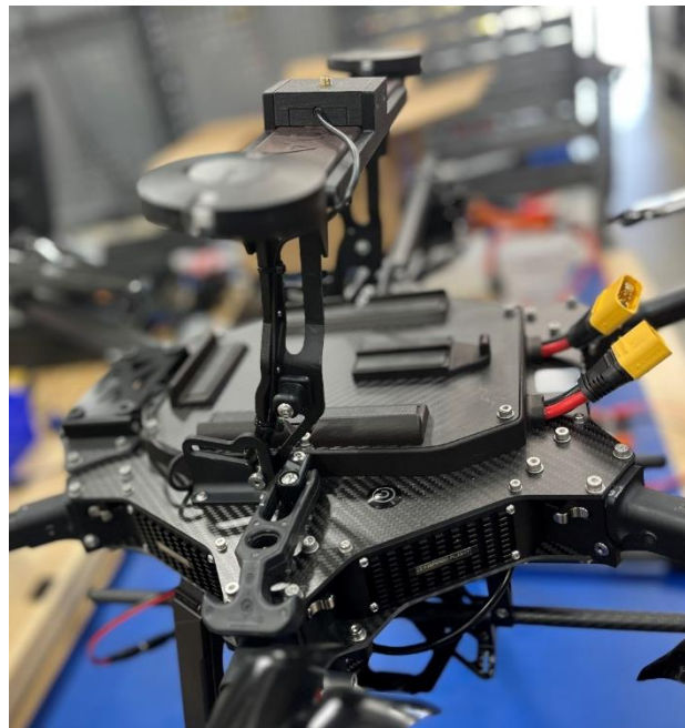
Figure 10. Attach the cable using zip-ties.
